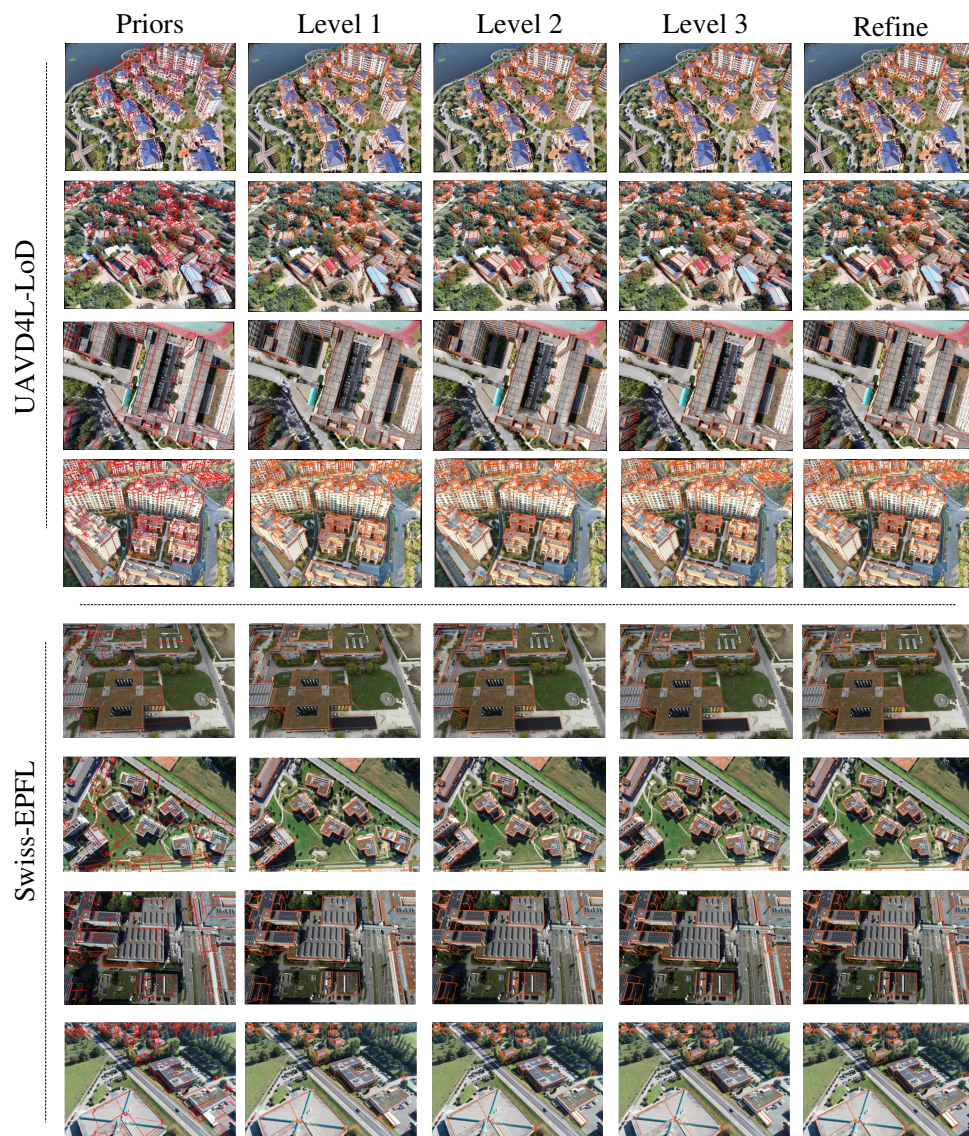
Figure 18: Visualization of predictions at different levels. Based on the predicted poses at each stage, we can obtain 2D projected wireframe and overlay them on the query image to check the accuracy of the poses. It can be observed that as the levels progress, the projected wireframes gradually align with the edges of the buildings. Please zoom in to see the details of the alignment.
