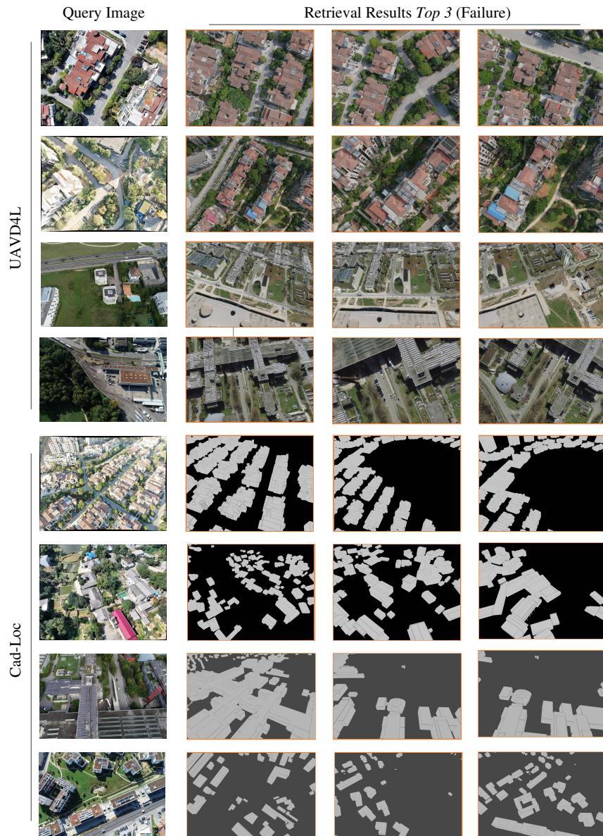
Figure 13: Failure retrieval cases of baselines. Even with narrowed searching scopes, the retrieval phase still suffers from issues such as repetitive textures and cross-modal challenges.
